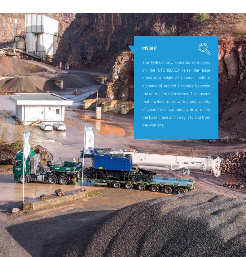
The GTC-1800EX is optimized for transport. The base crane is transported to the site on a low-bed truck, the crane components separately on several standard trucks. This means that separate driving permits are not required in most cases. This also means that the GTC-1800EX can get to the worksite faster – and get to work on lifts that would not be feasible otherwise.
