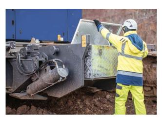
Sufficient space: the lockable aluminum box with a volume of 250 liters is intended for tools and personal items. Chain slings are kept in another large, open box.
