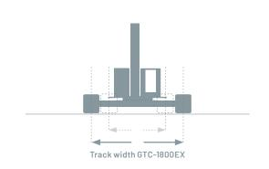
The track width is continuously variable, symmetrical and asymmetrical, within the range of 3.5 to 6 meters
